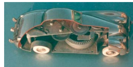
This is a special cut-away demonstration Prämetta model revealing the quality clockwork motor for which these models were famous. The car is still capable of operating perfectly. It can automatically follow different courses. These German cars were made in Cologne at the end of the Second World War.
