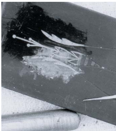
Fig 5. Marble clocks are often engraved with Greek style patterns which were originally decorated with a gold paint. They can be repainted or, as in the illustration, filled with gold wax. Method: Rub a hard, gold wax crayon across the pattern (as shown) until the pattern indentation is filled. With a sharp, flat piece of wood (a sliced cocktail stick is shown) scrape across the pattern until only the wax in the pattern indentation remains. Finally, rub hard with a soft cloth to polish. The illustration shows the various stages.
