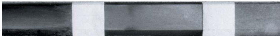
Fig 4. This piece of slate, originally in poor condition, has been sanded and then divided into three sections. One section has been left untouched (extreme right), one section has been waxed (unstained beeswax - centre section), while the third section (extreme left) has been treated with Zebo grate blacking before waxing.
