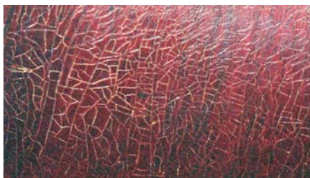
Fig 3. This Mahogany French polished veneer has crazed with age, probably from the heat of a coal fire. It is not difficult to correct, though some may prefer to accept it as part of the patina.
