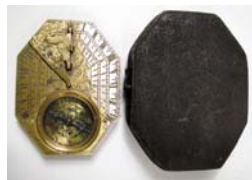
18thC Butterfield-type sundial compass, bird gnomon engraved with foliage and latitude scale of 45-60 degrees, compass with blued iron needle, underside of the horizontal plate engraved with latitudes of 16 English and Irish cities and towns, original fish skin covered case, 6.3cm. Sworders, Stansted Mountfitchet. Apr 05. HP: £680. ABP: £799.
