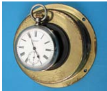
White metal keyless pivoted detent pocket chronometer with enamelled Roman dial, subsidiary seconds and blued steel hands, free sprung movement, cut bi-metallic compensation balance and blued steel spherical spring, signed Henry Capt, Geneve, no. 20330, associated brass bulkhead case. Gorringes, Lewes. Mar 04. HP: £1,500. ABP: £1,764.
