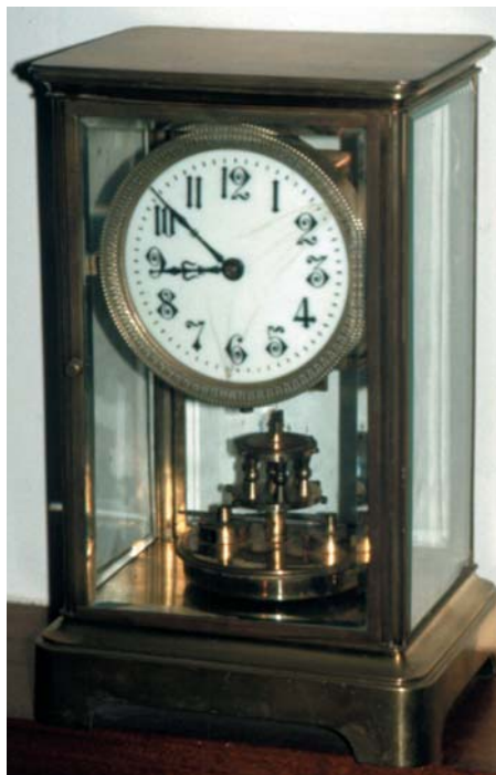
Fig 6. An Anniversary Clock by Gustav Becker in classical brass four-glass case. This example, late nineteenth century, is older than the ones normally found as may be seen by the movement fixing and the screwed disc pendulum (Ref. Anniversary Clocks, Shire Album No.331).
