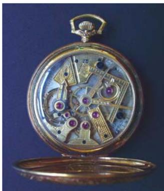
*Dudley Watch Company of Pennsylvania watch. View of movement showing working tools.*
