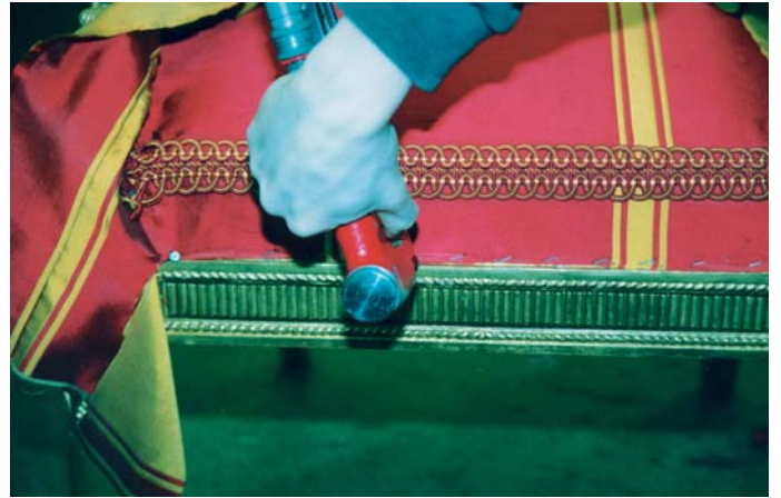
A single blow of the stapler and the fine pins of the staples are driven home with less damage to the frame.
