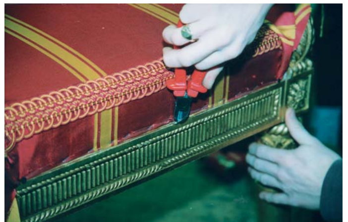
Use of staple remover to enable staples to be taken out without damage to the frame. Particularly important for gilded chairs.
