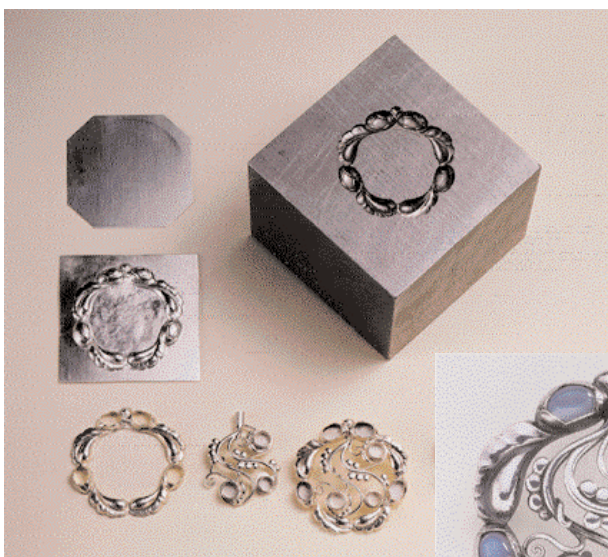
Die punch, matrix, unfinished parts and completed brooch. Cast iron, silver. And inset brooch designed by Georg Jensen 1914. Silver and moonstone.
